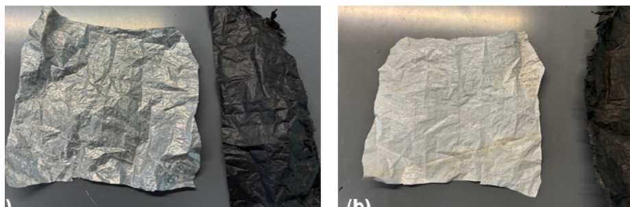
Figure 4. Plastic mulch films examined in furnace experiments: white/aluminized polyethylene and black polyethylene.
